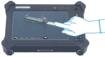
Touch screen monitor (target selecting is done by touching image on display)
