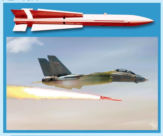
AD- 40A is designed as an air to air guided missile for interception of airborne targets in medium range. It is designed for F-14 aircraft and it is possible to be installed on the other types of aircraft.
