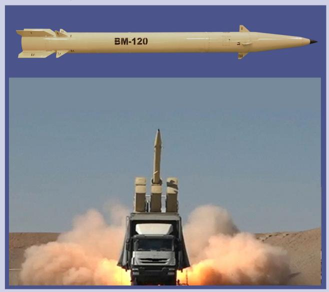
BM-120 is a single stage surface to surface ballistic solid propellant missile with blast warhead which is designed to destroy the enemy gathering points, command centers, missile sites, ammunition dumps, bases, military building, important centers & airports.
