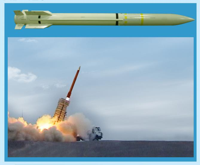
AD-120 missile weapon system is a high range and altitude surface to air defense system. It operates in all weather conditions and it is able to catch the target from any surveillance radar system. The system is designed for interception of advanced tactical and strategic aircrafts, UAVs and helicopters.
