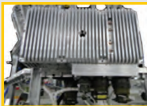
A view of processor, sampling, signal generation and storage subsystems of the SAR payload
