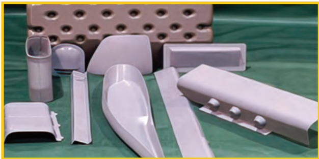
Part samples produced in vacuum forming method ◀
