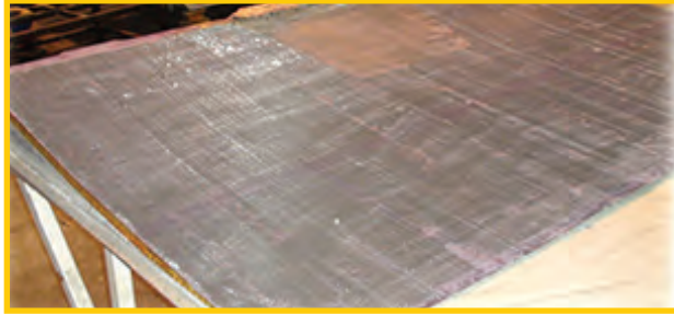
Reconstruction of Boeing-747 finalized spoiler
