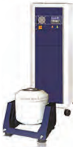
► Instant acceleration, mechanical shock and vibration tests stand
