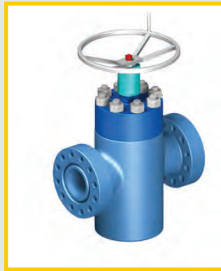
► Lower master gate valve BTM 11"-5K, top 9"-5K, 6-3/8" bore 5000 psi
